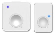
Power On: The blue LED indicator blinks once every 4 seconds.Operation: If the Logger is powered off, long press (over 1.5 seconds) the button to power on GPS Logger.
