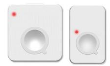
Power Off: The red LED indicator blinks once.Operation: If the Logger is powered on, long press (over 1.5 seconds) the button to power off GPS Logger.
