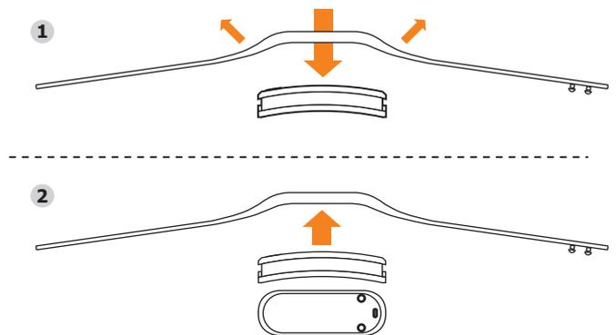
1. Spread open both bands with the screen facing up, and press down the screen with your thumb until the core comes off the wristband.
