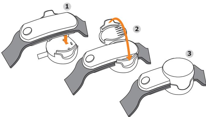
To charge your Q-Band X, place it in the charging box at the other end of the USB cable. Close the box afterwards, and make sure the Q-Band X is securely covered. Plug the USB connector to either a PC or power adapter to start charging.
